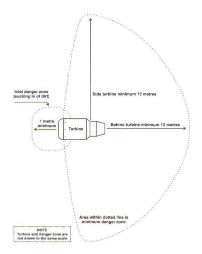
As can be seen from the diagram, the "safe" area near an operating turbine engine is in front of it and at least 1 metre away from the engine's inlet. Since Club rules require that turbines should have their outlet pointed away from the pits area when being started this will naturally place other occupants of the pits within the "safe" zone - so please don't undo that good work by moving round to stand alongside or behind the engine when it is running.
