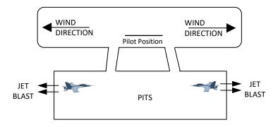
3. All gas turbine powered aircraft whose engines are being started must be positioned such that the jet tail pipes are pointing away from the pits, flight line, and runway.
